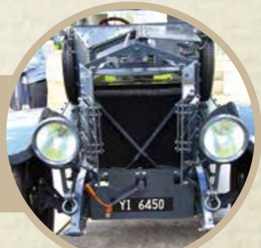
The added features of the Mk Ia including thicker radiator and electric lights.
